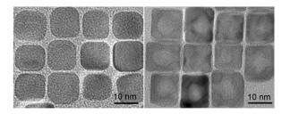
**Efficiency simplified**: A synthetic strategy has been developed to prepare single-crystalline hollow Pd/Pt nanocubes (right, see picture; left: nanocubes). Compared to the solid Pd/Pt nanocubes of similar
