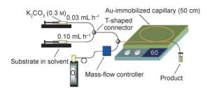
Golden capillaries: A gold-immobilized capillary column reactor allows oxidation of alcohols to carbonyl compounds using molecular oxygen. These capillary columns (see picture) can be used for at least four days without loss of activity.
