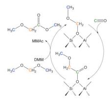
Carbonylation gets a phase lift: The usual liquid-phase, high-pressure processes for carbonylating formaldehydes are avoided in a novel vapor-phase reaction. Using an acid zeolite (Faujasite) at near-atmospheric pressure dimethoxymethane (DMM; the dimethyl acetal of formaldehyde; see scheme) is carbonylated to produce methyl methoxyacetate (MMAc). This approach provides a new route to ethylene glycol under mild conditions.
