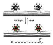
Dotting the i's: Stimuli-responsive optoelectronic devices are formed from the title transistors functionalized with photoactive quantum dots. The p-type semiconducting tubes show a fast current decrease under UV irradiation and reversibility when the UV irradiation is switched off. In contrast, ambipolar tubes show mirror-image photoswitching effects when negative and positive gate bias voltages are applied.
