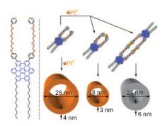
The assembly line: Hexabenzocoronene amphiphiles appended with pyridyl-terminated triethylene glycol side chains, in combination with trans-[Pt(PhCN)2Cl2], lead to the formation of graphitic nanotubes. The structural features and dimensions of the nanotubes depend on the assembly conditions. A platinum(II)bridged cyclic dimer having two HBC units self-assembles into a nanotubular structure.
