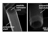
Breaking the mold: Self-assembled peptide nanowires were used as a template for the synthesis of hollow polyaniline (PANI) nanotubes (see scanning electron microscopy images). The thickness and the morphology of the PANI nanostructures could be controlled readily either by varying the reaction time or by applying multiple PANI coatings.
