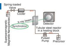
A general solution: In situ synchrotron X-ray scattering in a high-pressure pulsed injection reactor (see picture) shows that magnetite nucleation and growth are temporally separated. Gram-scale crystalline, pure phase, superparamagnetic magnetite nanoparticles were synthesized without surfactants in supercritical water in less than one hour using a laboratory-scale continuous-flow reactor.
